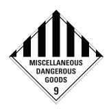
Figure 2: Li-ion batteries are classified as a Class 9 Dangerous Good
