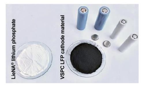
The (patents pending) processes that were used recovered the lithium from the waste materials as lithium phosphate ('LP'). The recovery of lithium from spent batteries harnessed cutting-edge technology designed for the recycling industry, while, for the lithium chemical industry, the technology provides a direct path to the production of LFP batteries, right now the fastest growing sector of the industry.
